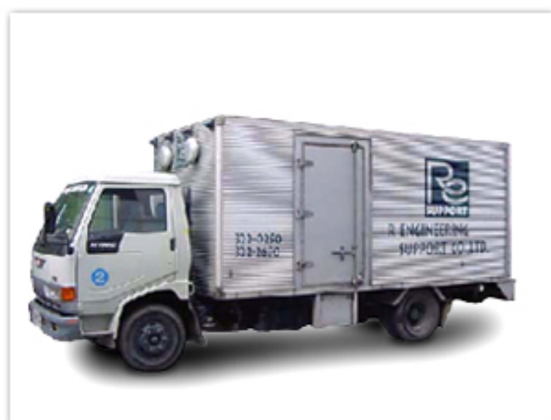
"Micafil-Switzerland" 4000 Litre/Hour Oil Treatment Plant Mobile
