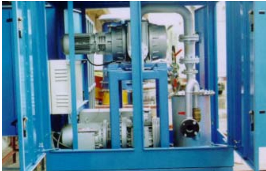
Rotary Vane Vacuum Pump Combined with Roots Pump complete with Pirani Gauge
